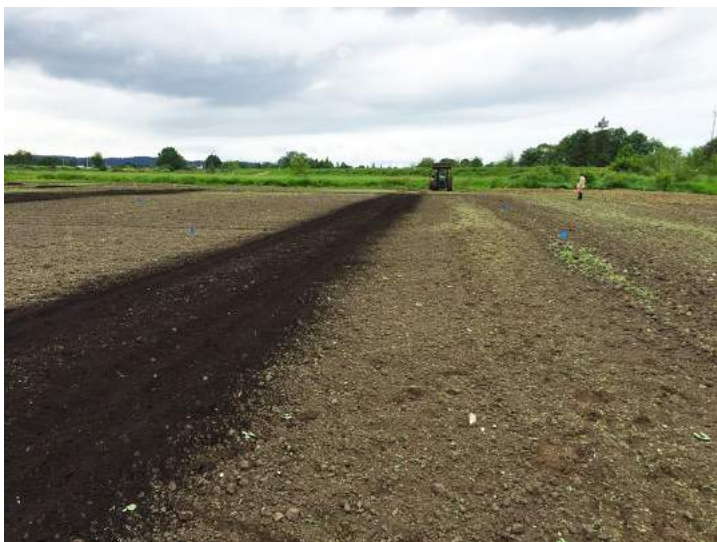
Figure 6. Spreader load calibration method. Determine the area spread from the length and width of the band. Photo by Andy Bary.
