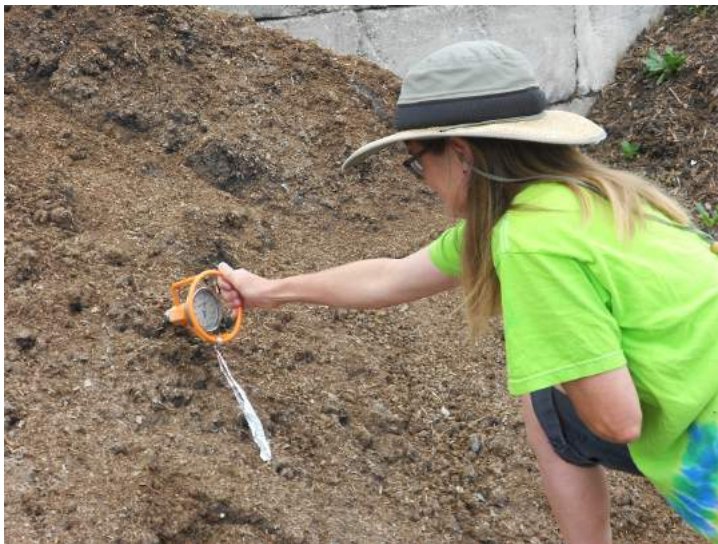
Figure 7. If you compost manure on farm, monitor temperatures daily during active composting to document meeting time and temperature standards for pathogen kill. Photo by Andy Bary.
