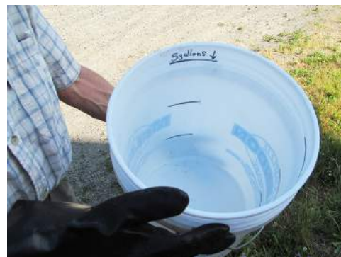
Figure 8. Calibrated bucket to use with dropped bucket method for estimating manure or compost bulk density. Photo by Andy Bary.
